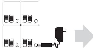
\* Each winder can work individually by using one AC power supplier.
